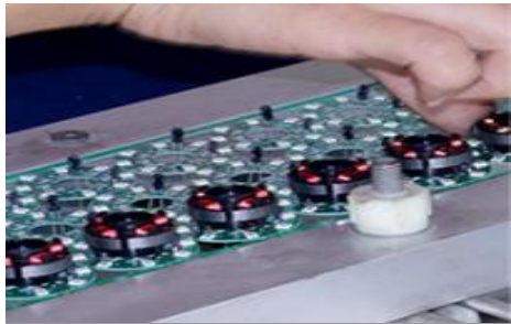
⑤ Motor and Motherboard assembled
